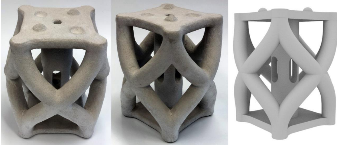
Figure 6: Geometric Sample Print, Front View (Left), Side View (Center), STL (Right)
